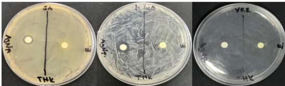
Figure 4. Investigation of the antibacterial activity of synthesised AgNP-THK compounds by disc diffusion method.
