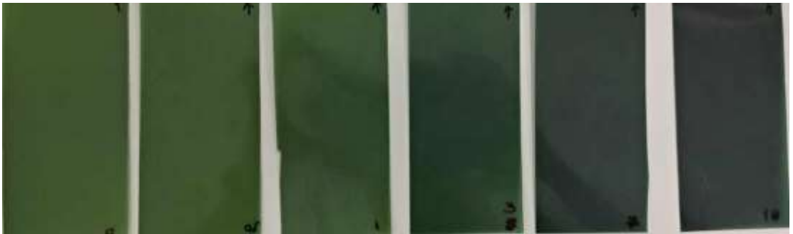
Figure.2 EBT3 film irradiated with different doses in QKUK
