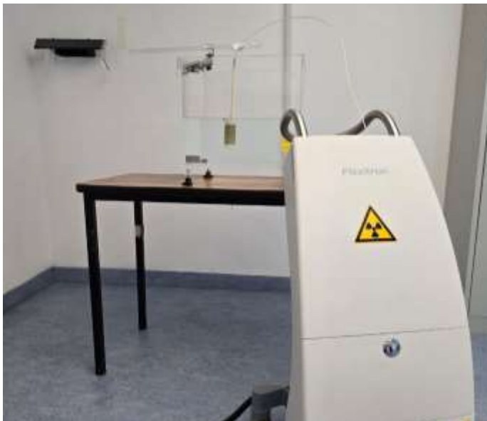
Figure.1 Experimental setup of HDR brachytherapy with a water mini-phantom, a vaginal applicator wrapped with Gafchromic film, and irradiation from Flexitron at QKUK-Prishtina
